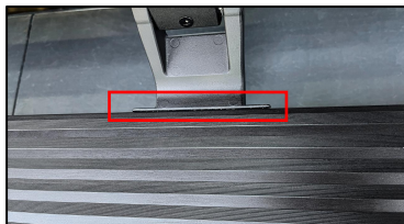
The panel is kept flush with the stent
