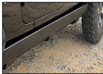
Step 2: Retract the panel and check if the front and rear gaps are consistent
