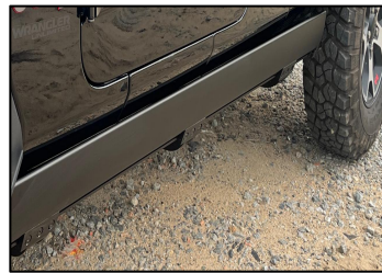
Step 2: Retract the panel and check if the front and rear gaps are consistent
