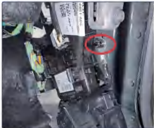
Negative cable: Inside right passenger trim panel, remove panel.
